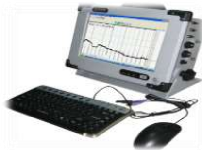
Plate 2 Specifications and Features of SDE-28S Digital Echo Sounder
